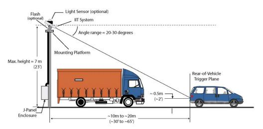
Note: Diagram applies to both front and rear plate geometries. With any configuration, the distance between camera and license plate must be in between 10m and 20m.
